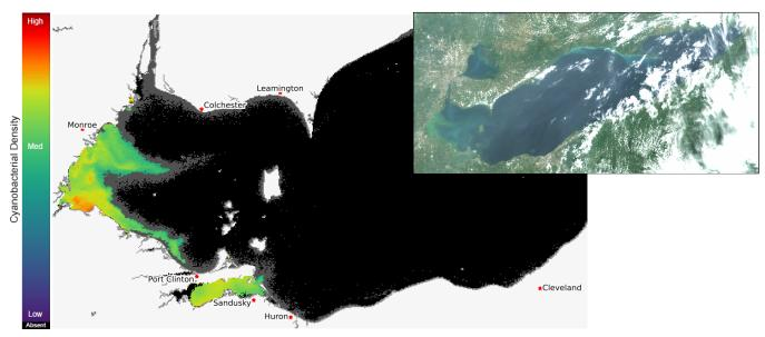
Current Lake Erie Sentinel-3 satellite imagery from the Ocean and Land Color Imager (OLCI) on Jul 25, 2023, showing bloom location and extent in the western basin. Grey indicates clouds or missing data. The estimated threshold of cyanobacteria detection is 20,000 cells/mL. Inset shows a truecolor image of the entire lake. Data derived from Copernicus Sentinel-3.
