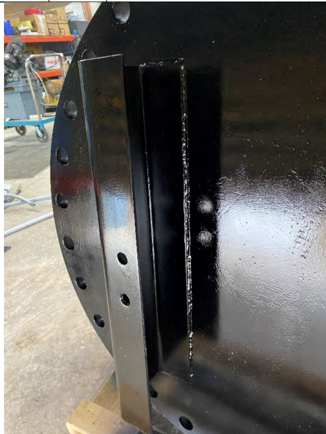
32. Blind Flange for East Tee in Valve Room – Channels Welded and Painted (2022-02-02)
