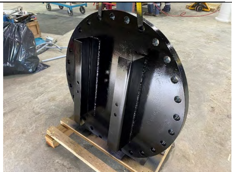
30. Blind Flange for East Tee in Valve Room – Channels Welded and Painted (2022-02-02)
