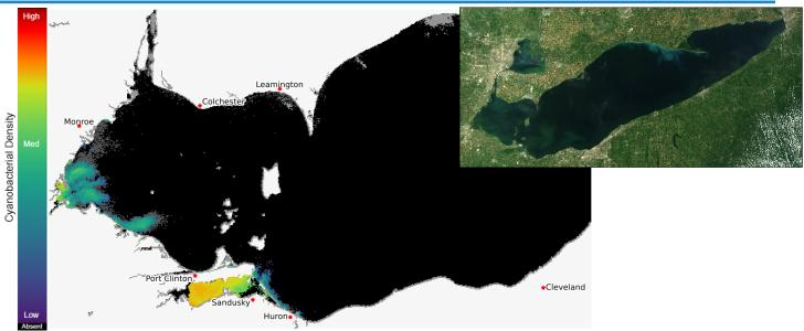
Current Lake Erie Sentinel-3 satellite imagery from the Ocean and Land Color Imager (OLCI) on Jul 23, 2025, showing bloom location and extent in the western basin. Grey indicates clouds or missing data. The estimated threshold of cyanobacteria detection is 20,000 cells/mL. Inset shows a truecolor image of the entire lake. Data derived from Copernicus Sentinel-3.
