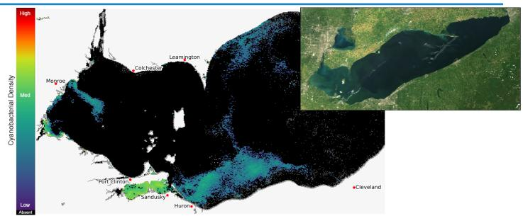
Current Lake Erie Sentinel-3 satellite imagery from the Ocean and Land Color Imager (OLCI) on Sep 12, 2025, showing bloom location and extent in the western basin. Grey indicates clouds or missing data. The estimated threshold of cyanobacteria detection is 20,000 cells/mL. Inset shows a truecolor image of the entire lake. Data derived from Copernicus Sentinel-3.
