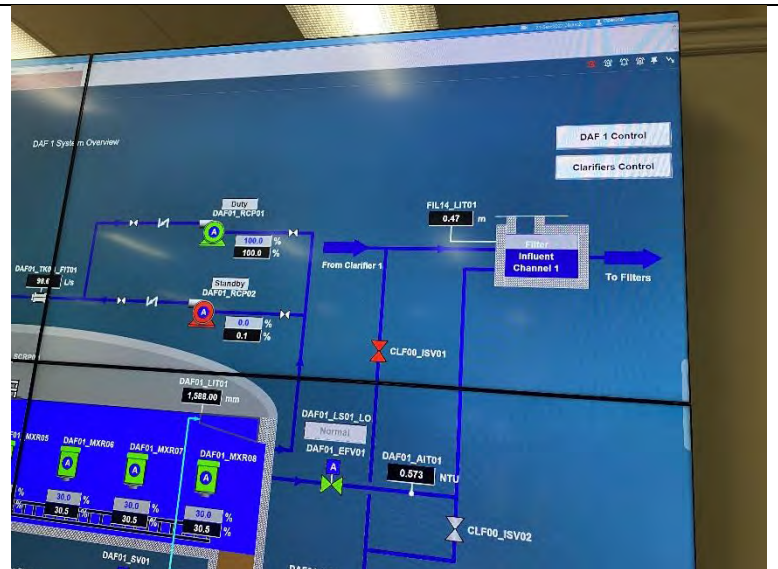
38. SCADA Screen: DAF No. 1 Overview (2022-09-21)
