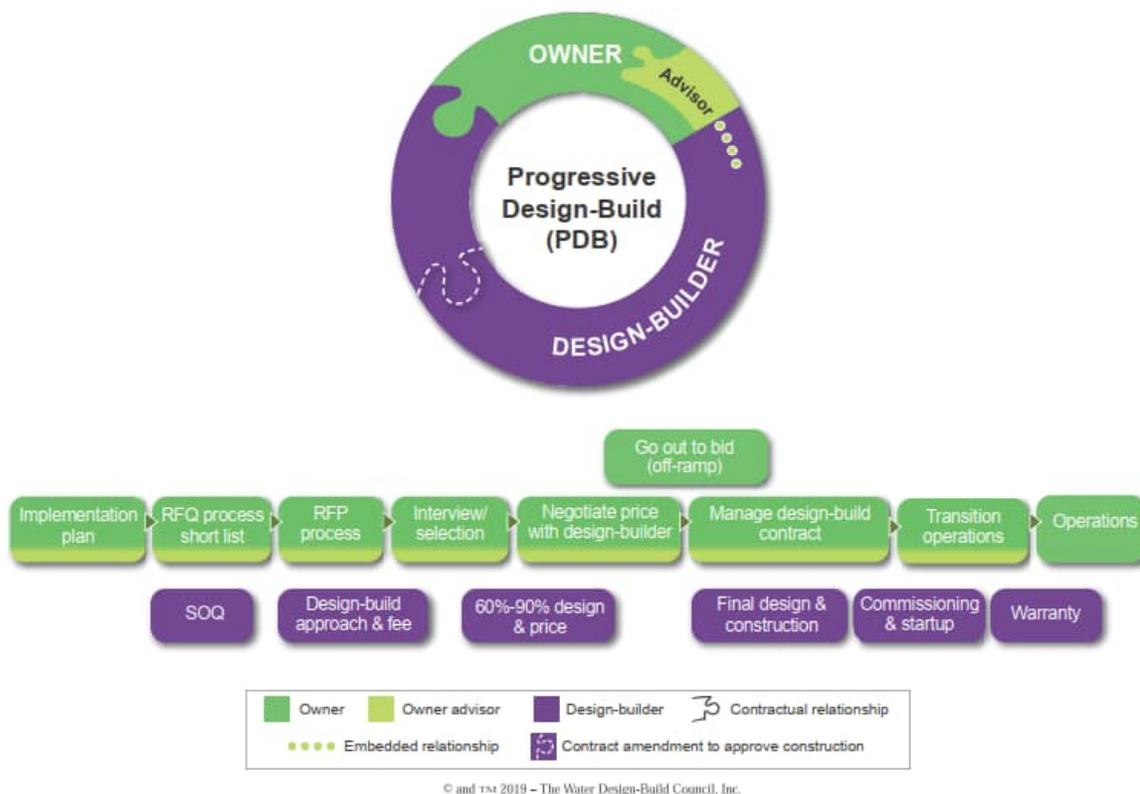
**Figure 3-5: Summary of the Progressive Design Build (PDB) Process** (Water Design Build Council, 2019)
